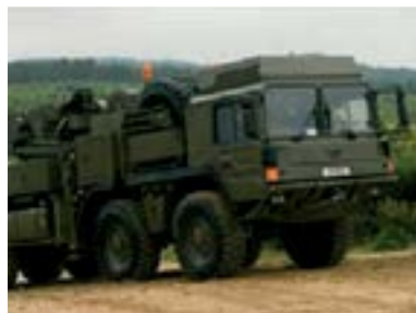
MAN Recovery unit with 600.2 crane
