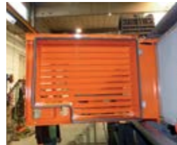
Side panel at the radiator
