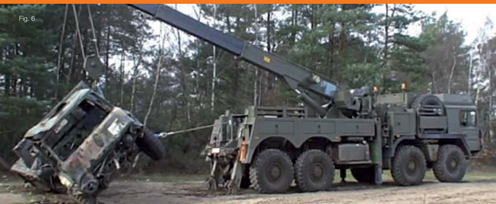
Fig 5 | SuperCompact with 'swing-away' towing pintle deployed. Demonstrated towing Warrior on Hollebhone system.
